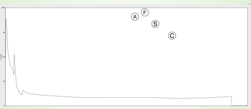
**Focusing**: 1000 V (1 min), 2000 V (1 min), 3000 V (6 min), 15 s interval time Sample: 2% ASFC Hb, 2% AESlyte 6-9, 70% MC 0.5 % Separation capillary **50x0.2 mm**
