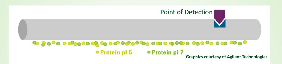
At the beginning of a CIEF run, the <u>whole</u> capillary (PFE coated fused silica) is filled with a mixture containing:
