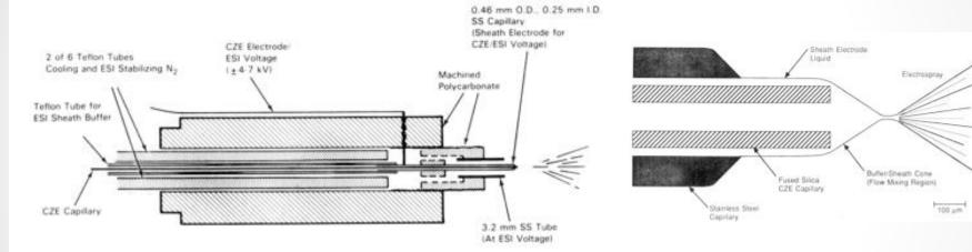
True Electrospray Liquid electrical contact Delivery of a sheath solvent to establish stable spray
