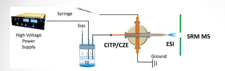
**Separation capillary**: FS 75x150 μm **Emitter capillary**: FS 200x350 μm, end etched with HF and orifice 50 μm **BGE**: 25 mM ammonium acetate, pH 4 **Sheath solvent and TE**:9/1 0.1 M acetic acid/methanol
