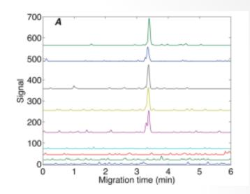
FS separation capillary 50x150 μm <u>Borosilicate</u> emitter capillary 0.75x1 mm, orifice 5 μm BGE 10 mM ammonium acetate, pH 5.5 Sheath solvent MeOH/0.1% formic acid Sample: short peptides
