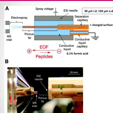
The high-sensitivity porous sprayer interface (A) schematic and (B) photograph of the prototype interface.
